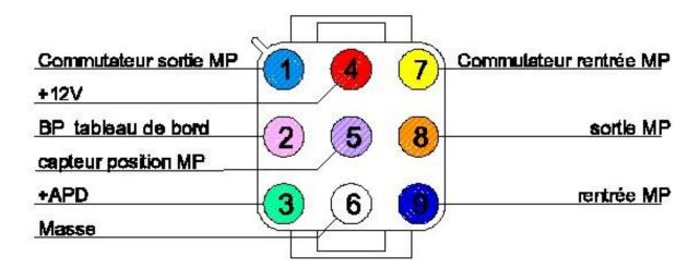
Selector switch extend step +12V Control panel press button Step position sensor + APD Earth
