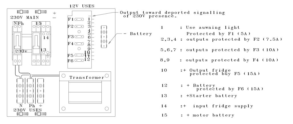
The clamp + has to be connected first to the battery.
